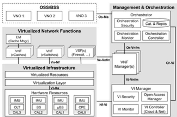
Figure 3: High-level CHARISMA control, management, and orchestration (CMO) plane
