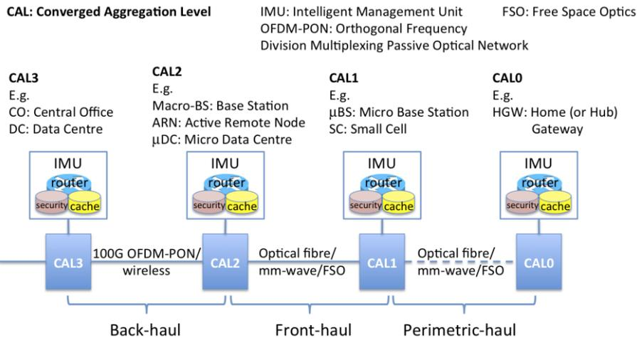
Figure 2: Physical layer description of hierarchical Converged Aggregation Levels (CALs)
